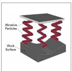
Our Scotch-Brite™ non-woven web binds together synthetic (nylon) fibres and abrasive particles to create a three-dimensional material. This web has a spring-like action allowing conformance to contours, edges and corners. What's more, our non-woven web is engineered to continually expose fresh abrasive to the work surface.
